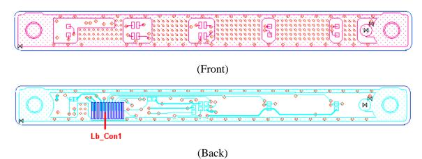
Figure B-5 LED Board layout (front/back)
